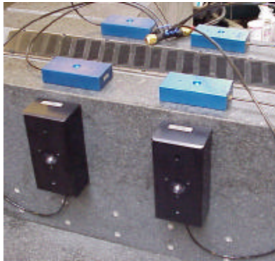
Figure A.4 Testing the vacuum system ensures that there are no leaks in the air system prior to squirting the epoxy. Notice the side bearing pads clamped to the way by the vacuum.
