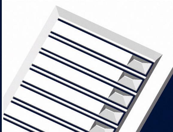
**Figure 4.8** Detailed view of the convex coupling array concept, notice the cantilevers and the KOH etched pyramids at the cantilever tips
