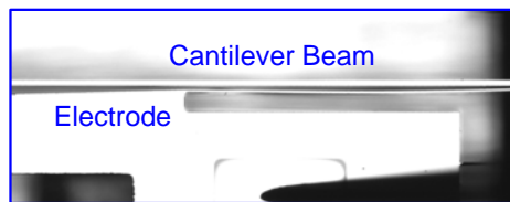
Device made using transparency mask and 10:1 Stepper
